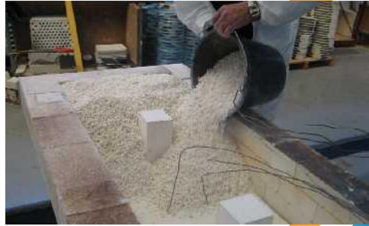
The heavier the material on kiln car more will be the gas consumption of the kiln. The heavier the furniture material, more the heat is utilized to heat up the car, which is of no use. The only useful heat is what absorbed by the product loaded on the car.
