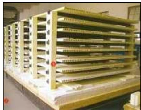
The specific gravity of the extruded cordierite batts is 2.57 – 2.66 with better thermal efficiency and thermal shock resistance and proven to reduce the gas consumption than the solid cordierite plates.
