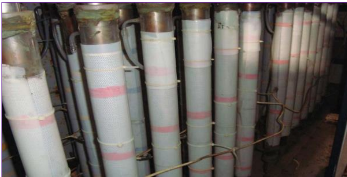
Figure 8.3: Inside View of an Ozonator (Supplied by Shivasu) installed at M/s Sri Vidya Industries, Erode
