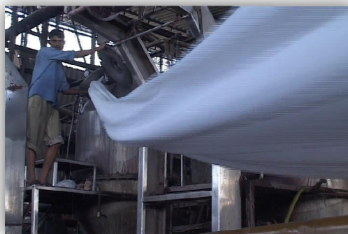
Batch washing in Jet Dyeing Machine
