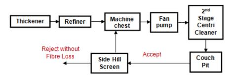
• Additional side Hill screen is placed in process, after the couch pit, to reduce continuous recirculation of pulp with direct supply to mixing (machine) chest after screening and fiber recovery with by-passing thickener and refiner.
