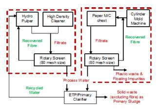
screening improved the process water quality which can be recirculated in the process loop. At the same time, the fiber recovery was improved which can be recycled in the process loop.
